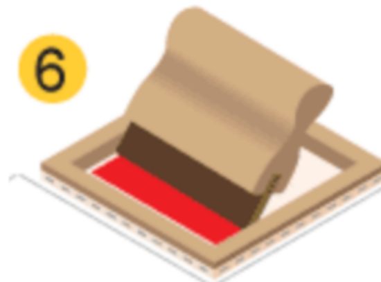
Step 6 – At a 45° angle using the squeegee passing the ink through the screen
