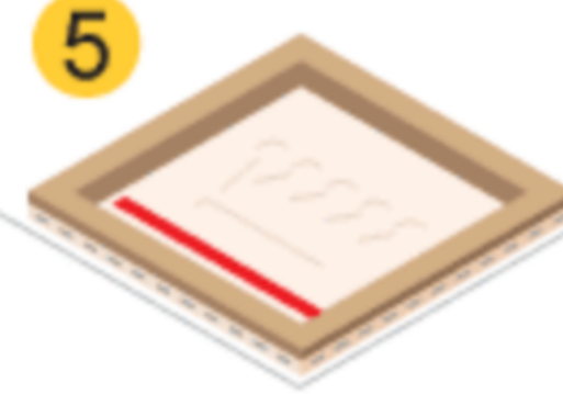
Step 5 - Adding a line of Ink along the edge of the screen (not too much ink)
