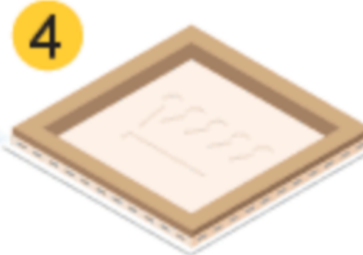
Step 4 - Placing stencil under the screen and above the page
